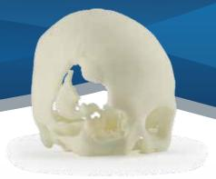
ABS-M30i is a high strength material well suited for the medical, pharmaceutical and food packaging industries. Parts manufactured with ABS-M30i material are biocompatible (ISO 10993 USP Class VI)<sup>\*</sup> and can be gamma or EtO sterilized. When combined with Fortus<sup>®</sup> 3D Production Systems, ABS-M30i gives you biocompatible Real Parts™ with excellent mechanical properties that are well suited for conceptual modeling, functional prototyping, manufacturing tools, and end-use-parts.
